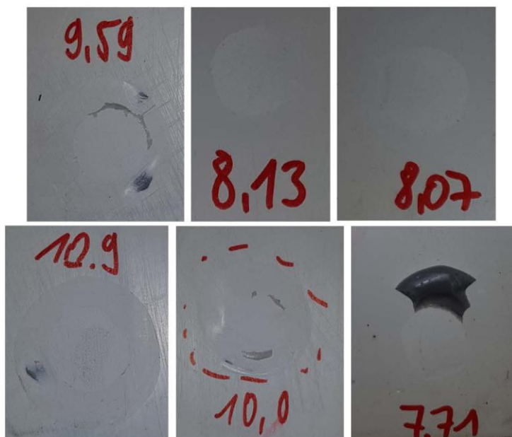
Figure 1 Failure patterns of the conditioned samples
